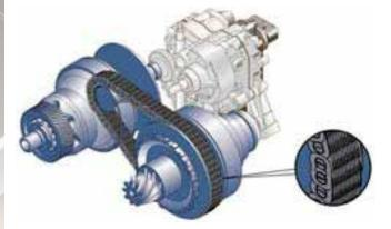
Traditional automatic transmissions use gears. CVT's don't have a gearbox but they operate on a pulley system that allows an infinite variability between highest and lowest gears with no discrete feeling of gear change.
