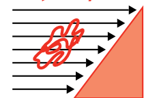
Polymer coil is squashed under temporary shear forces
