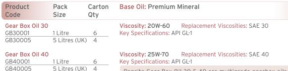
Penrite Gear Box Oil 30 & 40 are multigrade gearbox oils designed specifically for use in vehicles that originally used the same oil in the gearbox as was recommended and used in the engine. Many vehicles manufactured in the fifties and sixties specified engine oil for use in the gearbox. Whilst this was convenient, a proper gear oil was a better alternative. Both Gear Box Oil 30 & 40 meet the requirements of API GL-1.
