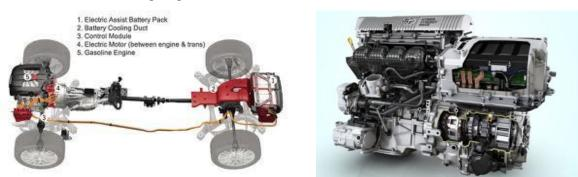
Most HEV's contain an internal combustion engine of similar size and performance to a standard combustion engined vehicle. This is needed for when rechargeable batteries that power the electric motors discharge. The combustion engine needs to be able to power the vehicle and recharge the battery packs for the electrical engine.
