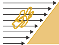
Polymer coil is squashed under temporary shear forces
